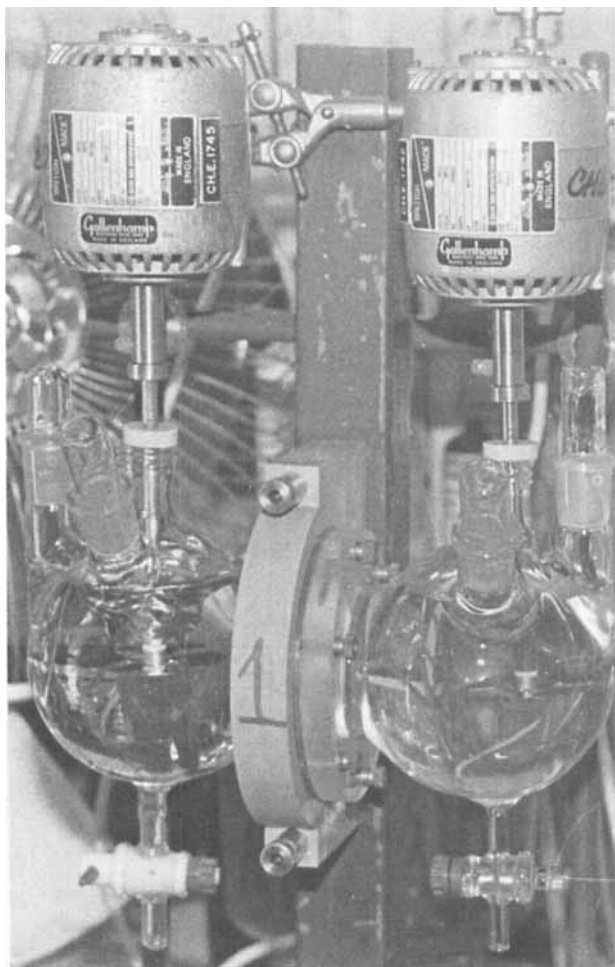
FIG. 4. Experimental apparatus for measuring the permeability.
